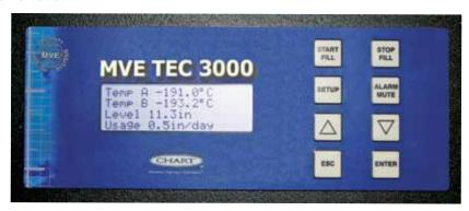
The TEC 3000 employs a variety of advanced features that enable the controller to monitor and control the environment inside a freezer with a high level of precision.
